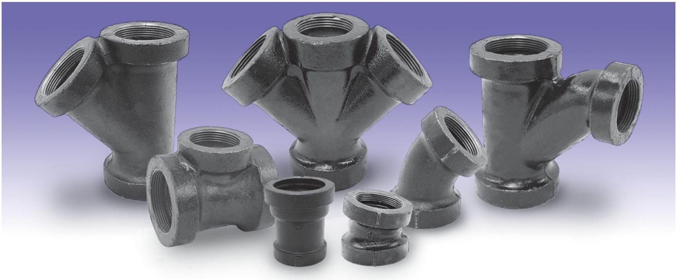
Anvil drainage fittings have sufficient sweep to allow free unobstructed flow. They are made with a shoulder of the same diameter as the inside of the pipe, in accordance with ASME B16.12, Type 1. Thus, continuous passage is created when the pipe is screwed to the shoulder, leaving no place for solid matter to collect and clog in the pipe.
